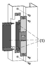
(1) If you order an ES2000X which has pre-drilled extension holes, 25 and 50mm extension lips can be fitted for extra wide door frames.
